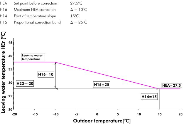
The minimum operating temperature for the **Aqu@Scop Advance DCI** for this application is limited by the parameter H23 to -20°C. The leaving water temperature is always below the limit and the appliance can operate with the boiler down to temperatures of -20°C. The boiler start-up temperature is determined by **Aqu@Scop Advance DCI**'s capacity (balance point).
