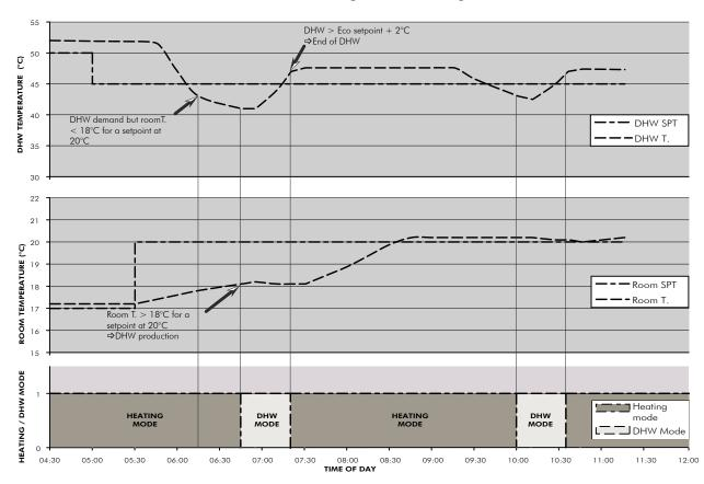
Heating and DHW mode operation in relation to scheduling, restart after night time running
