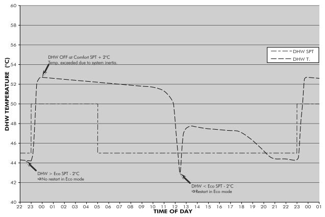
Off-peak input connected or daily scheduling with a restart at midday (Comfort between 0h00 and 05h00 in the morning and between 12h00 and 14h00, Eco the rest of the time), Comfort and Eco setpoints at 50°C and 45°C.
