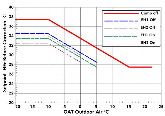
Example for default parameters with no correction for underfloor heating.
