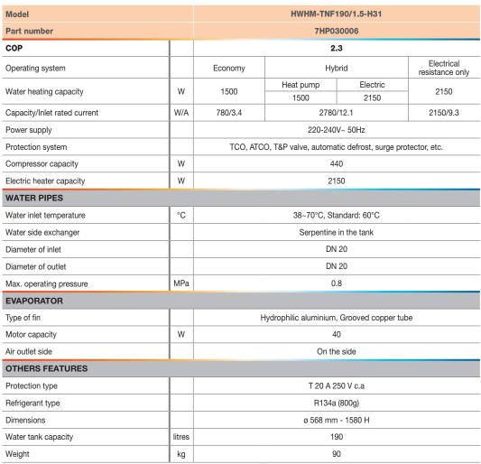
$Test\ conditions:\ outdoor\ temperature\ of\ 15/12°C\ (dry\ bulb\ /\ wet\ bulb),\ input\ water\ temperature\ 15°C,\ output\ water\ temperature\ 45°C.$
