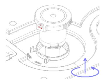
Once the UV has been replaced, go into the menu from the screen, select the "filter/UV maintenance" option, select "UV" and confirm the UV replacement.
