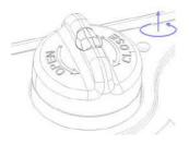
Remove the new filter from its packaging and insert it. Then turn clockwise to install.
