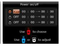
When the SPRING goes into standby mode, it will display the following screen in the display:
