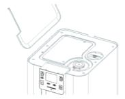
You will see the tops of two white filters on the right hand side. The filter is the one towards the back of your SPRING which a handle protruding from the top. Turn the handle anti-clockwise and pull the filter upwards and out.
