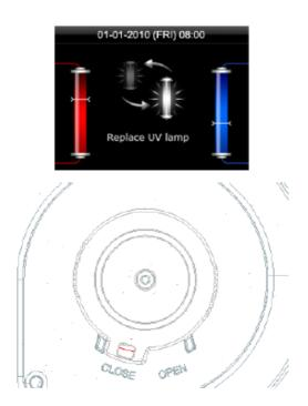
You will have been given a key when your SPRING was installed to release the UV filter. Put the key into the slot indicated above, release the latch to "open" and rotate the UV lamp counter clockwise. Pull the UV filter up and out of the SPRING.
