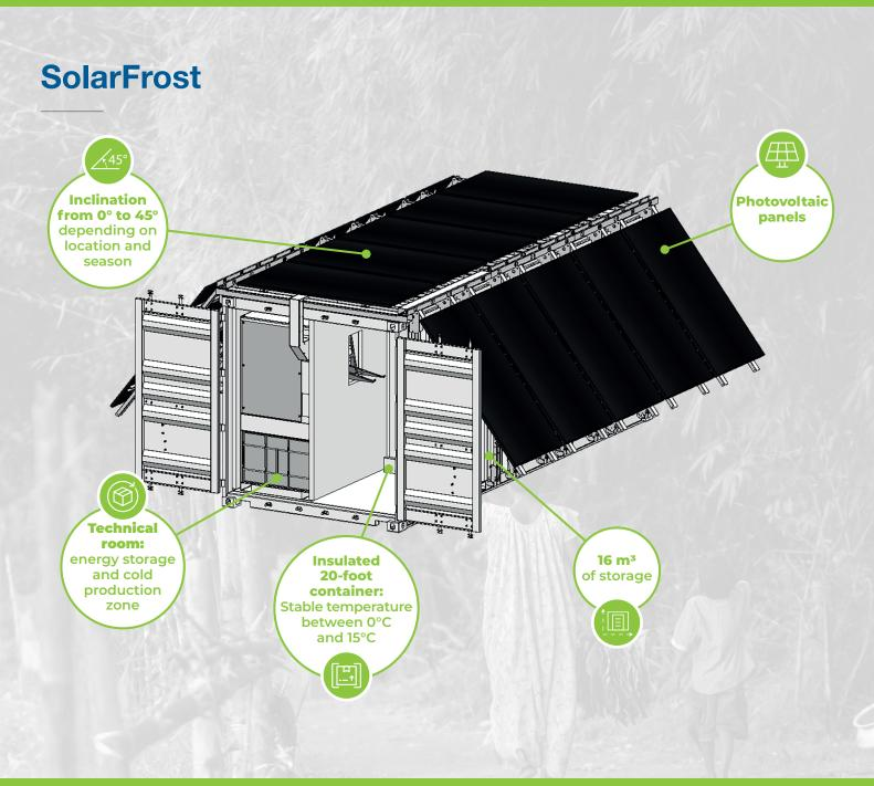
**SolarFrost, a simple principle:** the sun's rays are captured by solar panels and then transformed into electrical energy to power a refrigeration unit. Solar panels, batteries, cooling unit, inverter, all components are available in the SolarFrost, making it an off-grid and plug-and-play solution.
