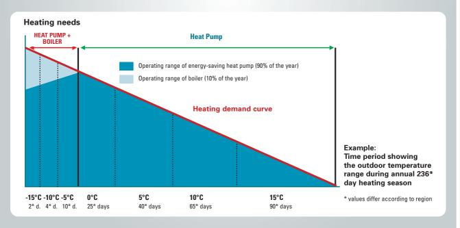
For 90 % of the heating season, the heat pump is able to fully meet the heating requirements and generates energy savings. For the remaining 10 %, the existing boiler provides the supplementary heating needed to ensure comfort in your residence. The system therefore enables you to cut your energy bill by up to 2/3, depending on the region.
