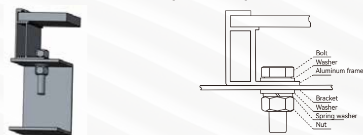
Figure 5 Bolt Installation of Mono-facial Modules
