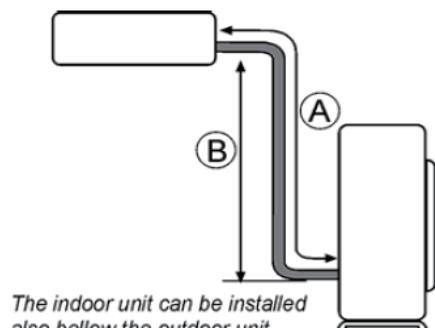
The indoor unit can be installed also bellow the outdoor unit.
