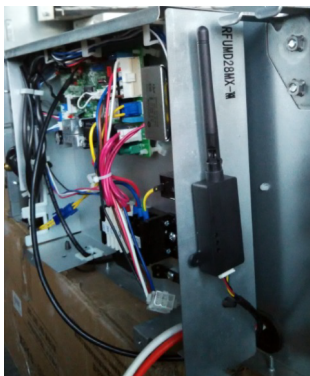
Installation Location Diagram of IDU Wireless Module
