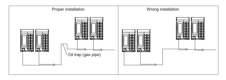
5. When the distance between outdoors(L1, L3, L5) is >2m, the oil trap must be set (upright gas pipe height≥0.2m), as the figure:
