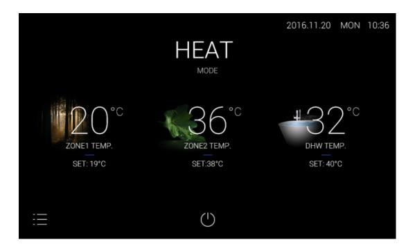
This controller can control all parts temperature of the split system, including Zone1, Zone2, DHW (Domestic Hot Water), and Pool.
