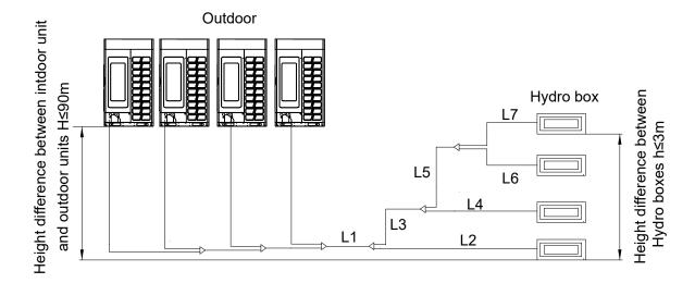
Allowable pipe length and height difference between indoor (Hydro box only) and outdoor units
