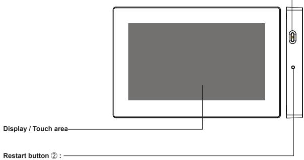
Press to restart controller. Check whether the controller chip is normal.
