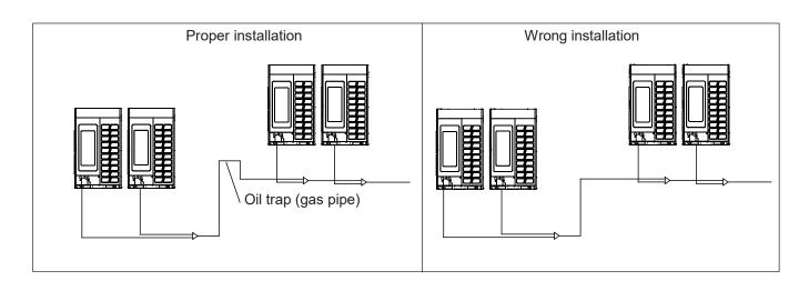
5. When the distance between outdoors(L1, L3, L5) is >2m, the oil trap must be set (upright gas pipe height≥0.2m), as the figure:
