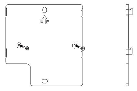
The hanging plate is placed in the direction of the illustration, where A/B is the location of the 86 cassette screws, and the C/D is the position of the 120 cassette screws. The pendant is fixed to the hole of the pendant, please pay attention to the UP direction.
