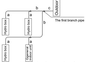
1. Pipe "a" diameter (between indoor units and branch pipe, diameter unit: mm)
