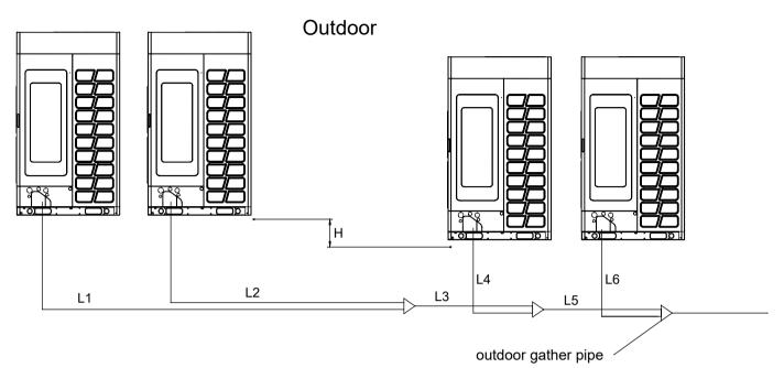
1. Pipe length between outdoor units and the first gather pipe should be≤10m; L1+L3+L5≤10m; L2+L3+L5≤10m; L4+L5≤10m; L6≤10m.
