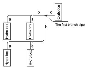
1. Pipe "a" diameter (between Hydro box and branch pipe, diameter unit: mm)
