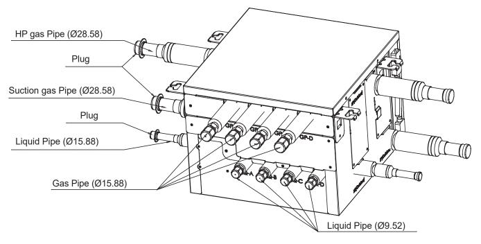
\*Note: Outdoor unit side: HP: HP gas pipe LP: Suction gas pipe LQ: Liquid pipe
