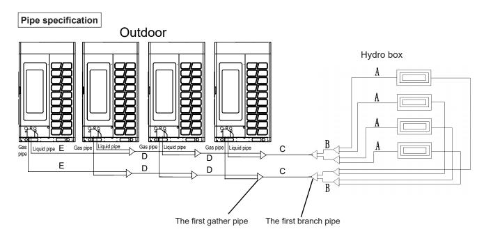
1. Pipe "A" diameter (between indoor units and branch pipe, diameter unit: mm )
