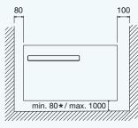
\* Warning! To facilitate the condensate drain from the service cap, however, it is advisable to install the unit at a minimum height of 300 mm.
