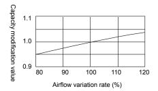
D. Capacity compensation suitable for total capability of indoor unit group
