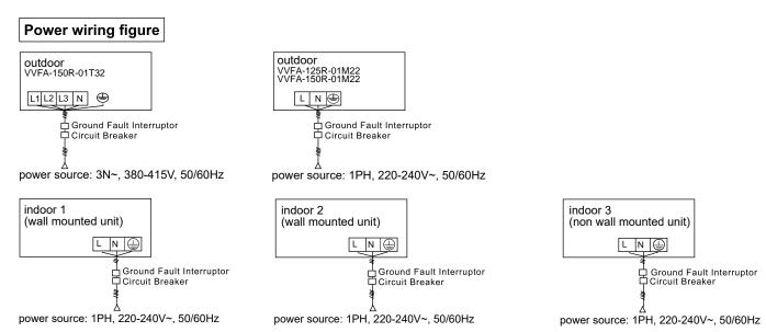
Indoor and outdoor use their individual power source. All indoors use one power source. Must install the leakage breaker and the over current breaker, or electric shock will occur.
