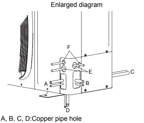
E:Power cord hole (with its own cable sheath)
