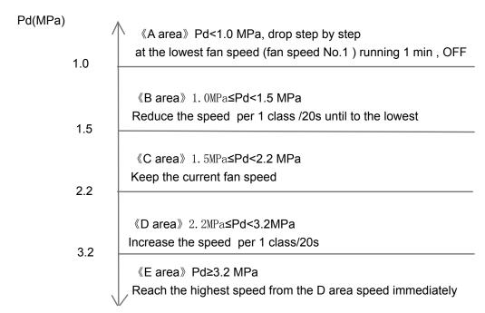
When startup the fan motor speed refer to the following:
