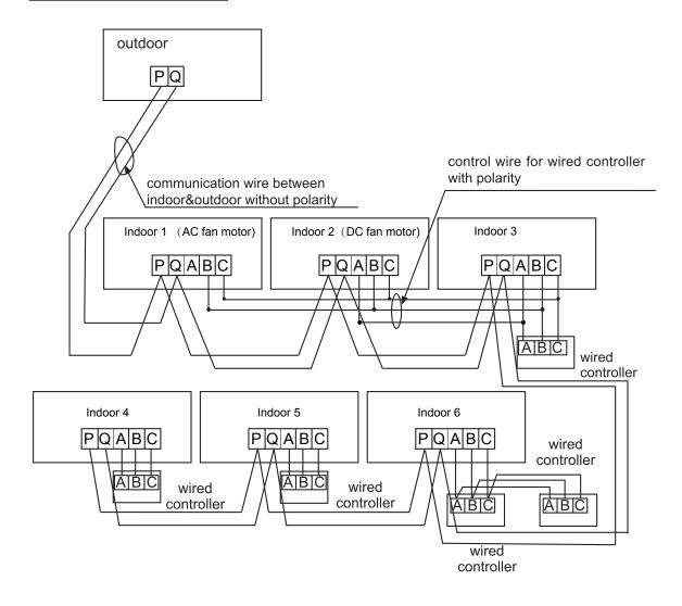
The master outdoor and all indoor units are in parallel through 2 non-polar wires.
