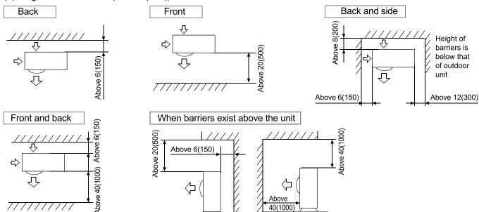
The top and two side surfaces must be exposed to open space, and barriers on at least one side of the front and back shall be lower than the outdoor unit.
