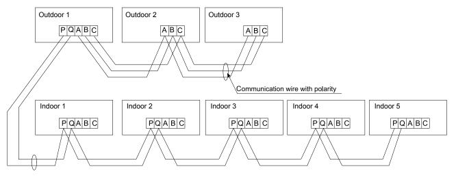
Outdoor units are of parallel connection via three lines with polarity. The master unit, central control and all indoor units are of parallel connection via two lines without polarity. The singal line between wired controller and indoor units are polarity
