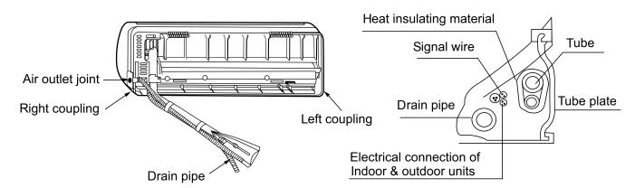
(4) Lead the connection tubing(liquid pipe and gas pipe) through the hole into the wall, or connect piping and wiring of indoor unit(check the number of wiring terminals of indoor and outdoor units and connect terminals with the same number and color), and then put the connection tubing and the connecting line through from the inside wall for the connection with outdoor unit.
