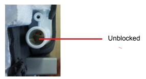
But for HVVA-070/050/045N-01M22 and HVVA-090N-01M22 indoor untis the middle of the left drain is blocked, so first need to knock off the middle of the blocking piece and take it out to avoid noise when the unit is running. Then install the drain pipe.
