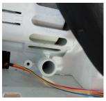
Step 2: Unplug the rubber plug on the drain hole on the left side of the unit
