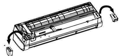
2. Remove 2 gaskets under the cross-flow fan. (used for HVVA-045~070N-01M22)
