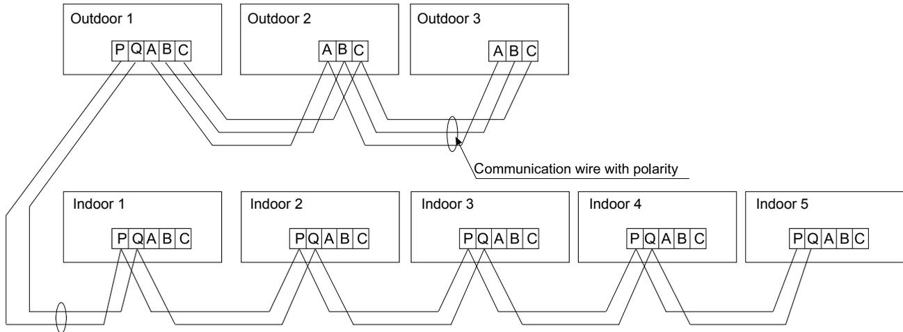
Outdoor units are of parallel connection via three lines with polarity. The master unit, central control and all indoor units are of parallel connection via two lines without polarity. The signal line between wired controller and indoor units are polarity
