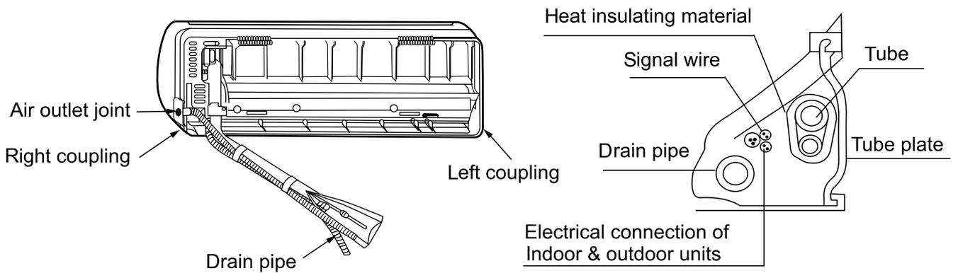
(4) Lead the connection tubing(liquid pipe and gas pipe) through the hole into the wall, or connect piping and wiring of indoor unit(check the number of wiring terminals of indoor and outdoor units and connect terminals with the same number and color), and then put the connection tubing and the connecting line through from the inside wall for the connection with outdoor unit.
