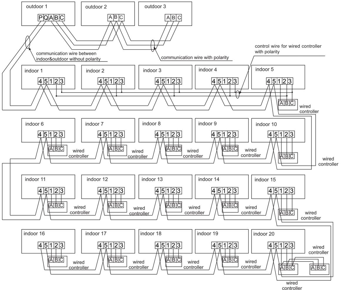
Outdoor units are of parallel connection via three lines with polarity. The main unit, central control and all indoor units are of parallel connection via two lines without polarity.
