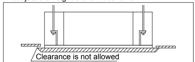
If the elevation level of the indoor unit and drain pipe are not affected, you can adjust the height of the indoor unit through the corner pore on the trim panel. Please keep the unit horizontal in the process of adjustment, or else water leakage is easy to occur.
