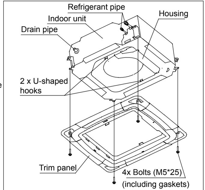
5) When tightening the four (4) bolts, please make sure there is no clearance between the panel fixing seat on the side of the indoor unit and the panel fixing seat on the side of the panel. That is to say: the bolts shall be fully tightened (see \* in the figure).
