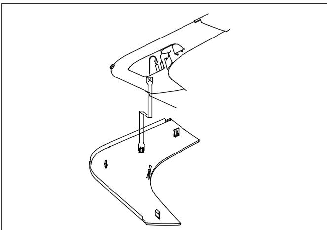
8) Installing the air-inlet grille.
