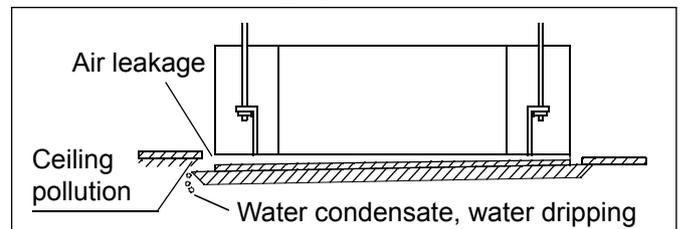
■ After tightening the bolts, if there is a clearance between the ceiling and the trim panel, please readjust the height of the indoor unit.
