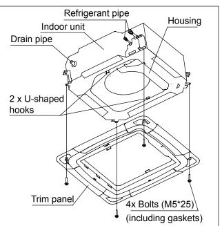
5) When tightening the four (4) bolts, please make sure there is no clearance between the panel fixing seat on the side of the indoor unit and the panel fixing seat on the side of the panel. That is to say: the bolts shall be fully tightened (see \* in the figure).
