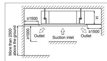
Space required for installation (unit: mm)
