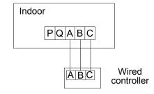
B. Two wired controllers control one indoor unit. Either of the wired controls can be set to be the master wired controller while the other is set to be the slave wired controller.
