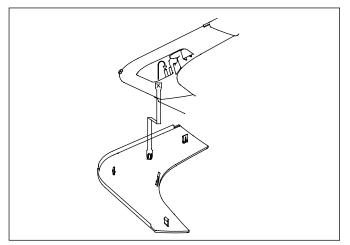
8) Installing the air-inlet grille.
