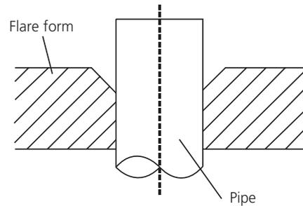
6. Place flaring tool onto the form.
