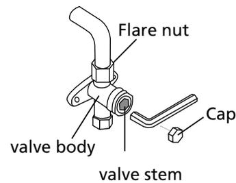
12. Using hexagonal wrench, fully open both the high pressure and low pressure valves.
