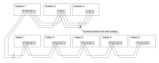
Outdoor units are of parallel connection via three lines with polarity. The master unit, central control and all indoor units are of parallel connection via two lines without polarity. The singal line between wired controller and indoor units are polarity
