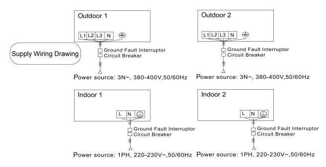
Indoor units and outdoor units should be connected to the power source separately. Indoor units must share one single electrical source, but its capacity and specifications should be calculated. Indoor & outdoor units should be equipped with the power leakage breaker and the overflow breaker.
