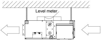
Choice of Blowing Wind from Blower (when using the high performance filter)
