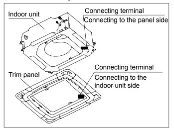
7) When the installation of panel is complete, please fix the four (4) angle trim panels.
