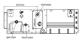
(a) Keep a gradient (1/50-1/100) of the drainpipes and avoid lobbing or curving.
