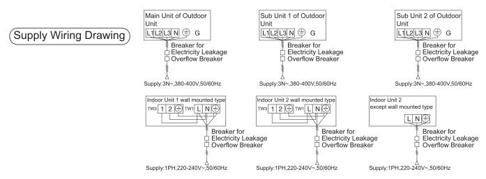
• Indoor units and outdoor units should be connected to the power source separately. Indoor units must share one single electrical source, but its capacity and specifications should be calculated. Indoor & outdoor units should be equipped with the power leakage breaker and the overflow breaker.
