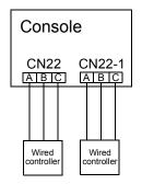
Master and slave controller setting method for RWV05, other controllers' setting method please refer to the controller manual
