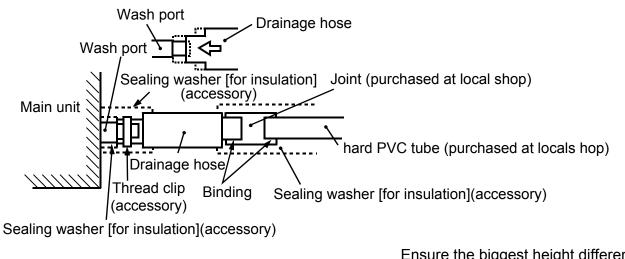
(d) When the laid drain piping is used for multiple equipments, the public piping should be lower about 100mm than the wash ports of equipments, as shown in the figure. Thicker pipes should be used for this application. Ensure the biggest height difference (about 100mm)
