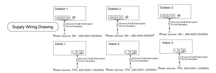
Indoor units and outdoor units should be connected to the power source separately. Indoor units must share one single electrical source, but its capacity and specifications should be calculated. Indoor & outdoor units should be equipped with the power leakage breaker and the overflow breaker.
