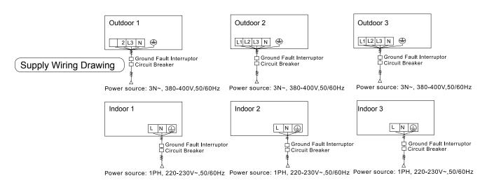
Indoor units and outdoor units should be connected to the power source separately. Indoor units must share one single electrical source, but its capacity and specifications should be calculated. Indoor & outdoor units should be equipped with the power leakage breaker and the overflow breaker.
