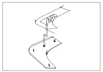
8) Installing the air-inlet grille.
