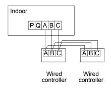
Master and slave controller setting method for RWV05, other controllers' setting method please refer to the controller manual
