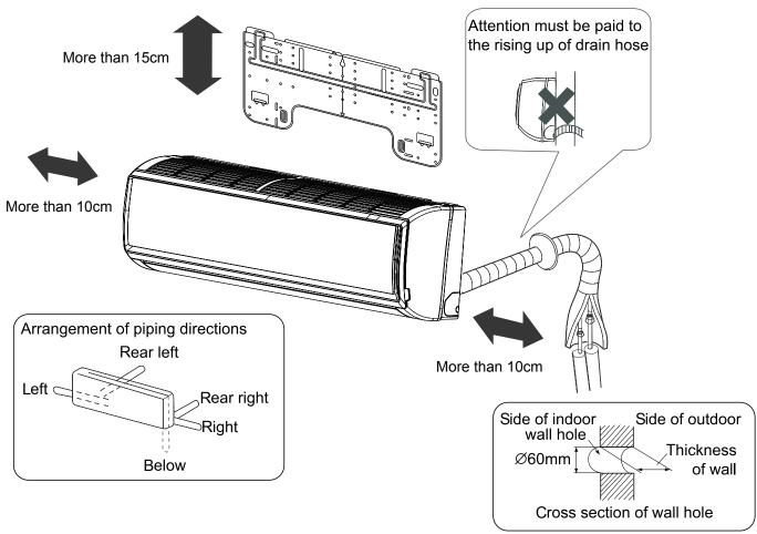
(1) Positioning Wall Pad & Locating Wall Holes
