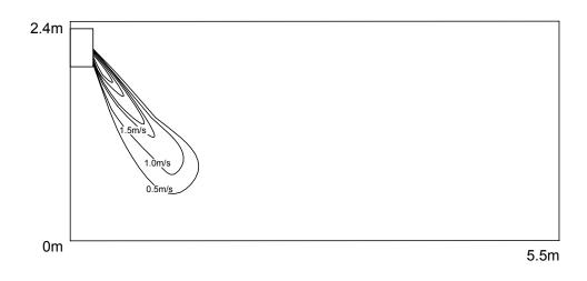
d. Cooling / Temperature distribution Blowy angle: 65
