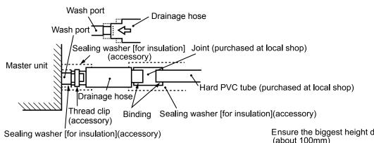
(d) When the laid drain piping is used for multiple equipments, the public piping should be lower about 100mm than the wash ports of equipments, as shown in the figure. Thicker pipes should be used for this application.
