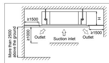
Space required for installation (unit: mm)
