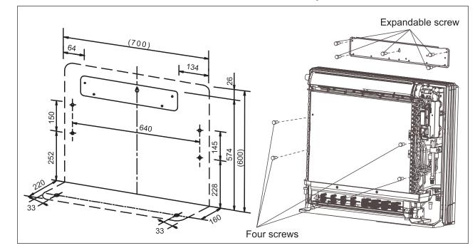
• Fix the wall board, then use four screws to fix the unit on the wall. As the figure shown.
