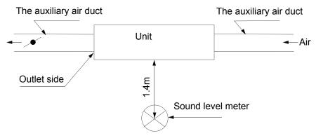
Testing position just below the central of the unit
