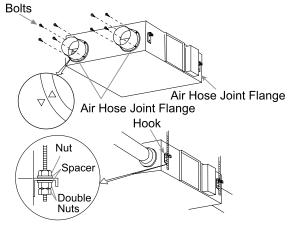
Installing air hose joint flange: fix four joint flanges with bolts.
