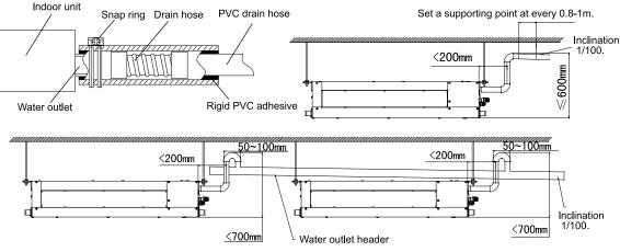
Multiple units use water outlet header to drain water into drainage ditch.
