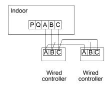
Master and slave controller setting method for RWV05, other controllers' setting method please refer to the controller manual
