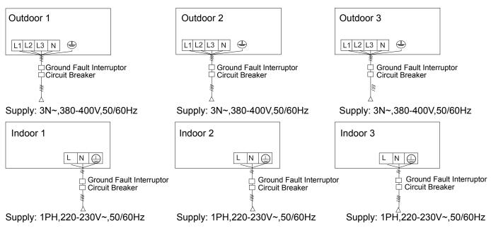
Indoor units and outdoor units should be connected to the power source separately. Indoor units must share one single electrical source, but its capacity and specifications should be calculated. Indoor & outdoor units should be equipped with the power leakage breaker and the overflow breaker.
