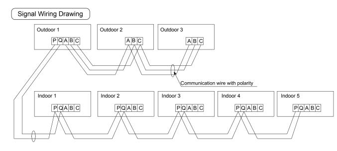
Outdoor units are of parallel connection via three lines with polarity. The master unit, central control and all indoor units are of parallel connection via two lines without polarity. The singal line between wired controller and indoor units are polarity
