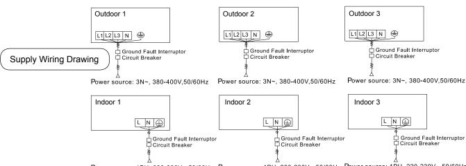
Power source: 1PH, 220-230V~,50/60Hz Power source: 1PH, 220-230V~,50/60Hz Power source: 1PH, 220-230V~,50/60Hz
