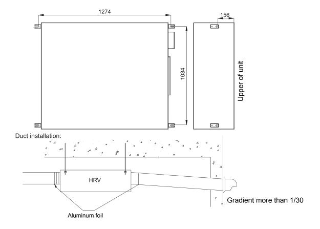
Install the two outdoor ducts at a certain gradient (no less than 1/30) to avoid the water flowing backward. Meanwhile the three ducts (two outdoor ducts, one indoor duct) all need the heat insulation material against the dew. Installation distance between air discharging hole and air inlet hole should be 3 times longer than duct.
