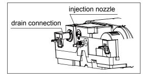
Confirm the sound of the motor: Confirm the sound of the motor of the drainage pump and meanwhile check the drainage.
