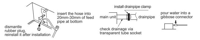
Before completing the electrical connection, a gibbose connector shall be installed on the drainpipe as to provide it with a water inlet port. Then, if any leakage exists in the piping, check it to make the water flow of the drainpipe smooth.
