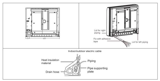
• Indoor/outdoor electric cable and drain hose must be hound with efrigerant piping by protecting tape. [Other direction piping]
