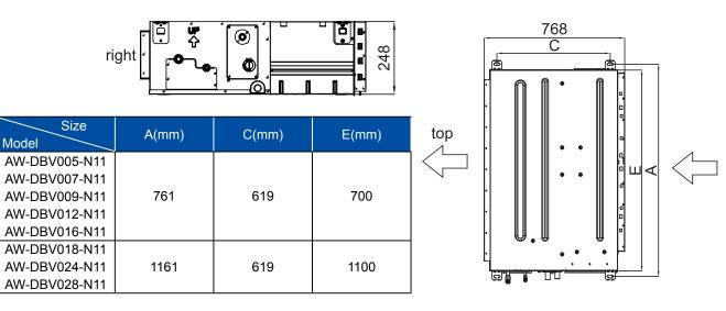
(2) If necessary, make a hole for installation and inspection on the ceiling. (used for the situation with a ceiling)For the size of the inspection hole on the ceiling, please refer to the above drawing.
