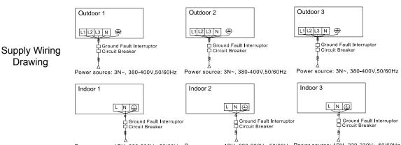
Power source: 1PH, 220-230V~,50/60Hz Power source: 1PH, 220-230V~,50/60Hz Power source: 1PH, 220-230V~,50/60Hz
