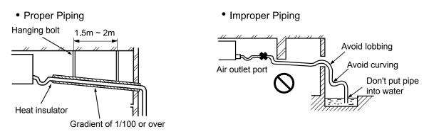
(b) When connecting the drainpipe to the equipment, don't apply too much force on one side of the equipment. Meanwhile, the piping should be positioned as close to the equipment as possible.
