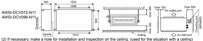
For the size of the inspection hole on the ceiling, please refer to the above drawing.
