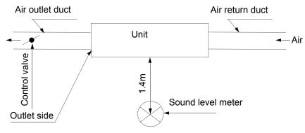
Testing position just below the central of the unit
