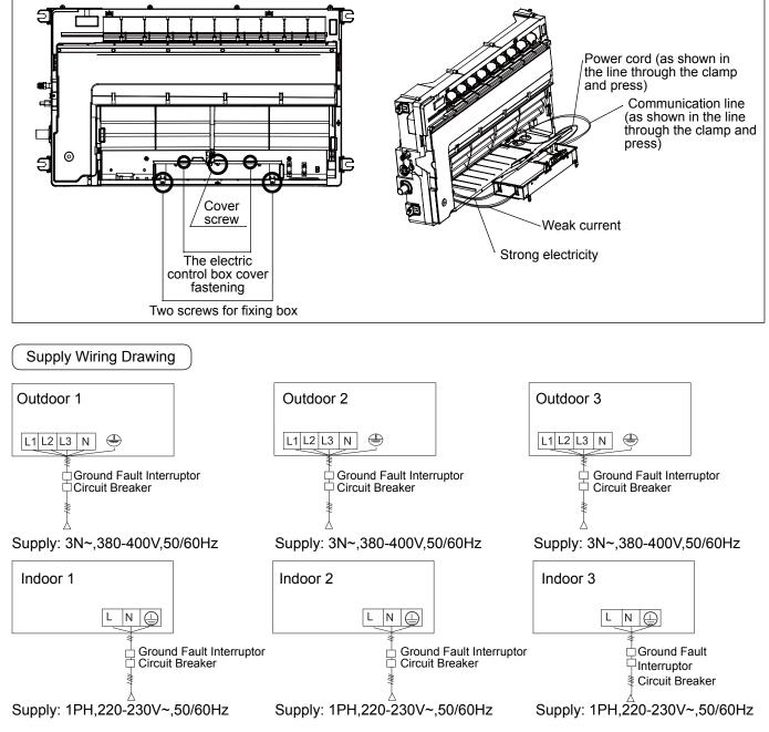
Indoor units and outdoor units should be connected to the power source separately. Indoor units must share one single electrical source, but its capacity and specifications should be calculated. Indoor & outdoor units should be equipped with the power leakage breaker and the overflow breaker.
