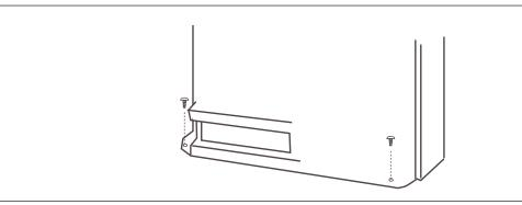
• Once refrigerant piping and drain piping connections are complete, fill the gap of the through hole with putty. Attach the front panel and front grille in their orginal positions once all connections are complete.
