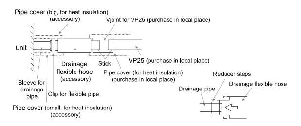
Make drainage slope down (slope is 1/50-1/100), and any part of drainage upheaval or cave in.
