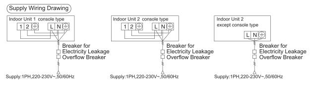
• Indoor units and outdoor units should be connected to the power source separately. Indoor units must share one single electrical source, but its capacity and specifications should be calculated. Indoor & outdoor units should be equipped with the power leakage breaker and the overflow breaker.
