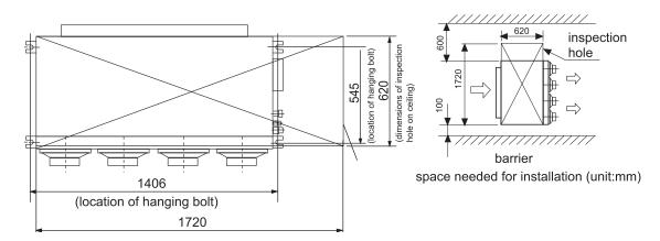
(2) If necessary, make a hole for installation and inspection on the ceiling. (used for the situation with a ceiling)
