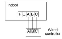
B. Two wired controllers control one indoor unit. Either of the wired controls can be set to be the master wired controller while the other is set to be the slave wired controller.
