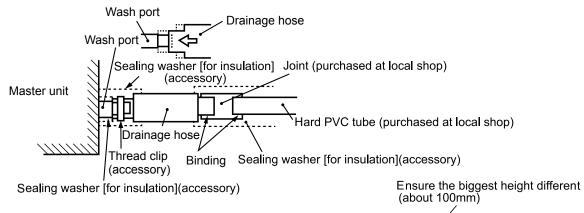
(d) When the laid drain piping is used for multiple equipments, the public piping should be lower about 100mm than the wash ports of equipments, as shown in the figure.
