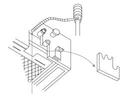
Insert the head of water supply pump into the hole beside the pump for about 50mm
