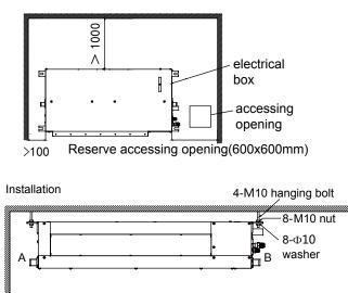
Please use the level meter, make sure the unit level be within 5mm; If drainage from A, ensure that B is slightly higher than A, in order to facilitate drainage; If drainage from B, ensure that A is slightly higher than B.
