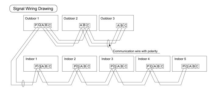
Outdoor units are of parallel connection via three lines with polarity. The master unit, central control and all indoor units are of parallel connection via two lines without polarity. The singal line between wired controller and indoor units are polarity
