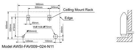
④ Installing Drain Pipe
