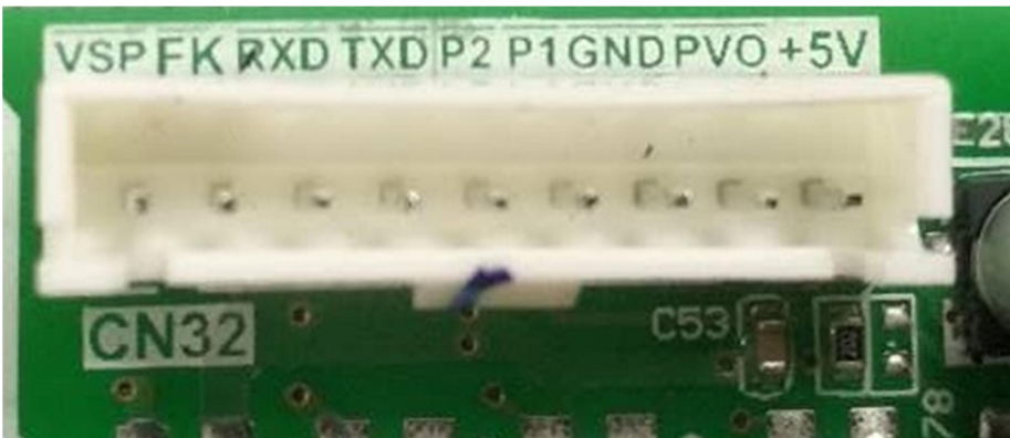
Figure 4-4.6: Connection port for inverter module
