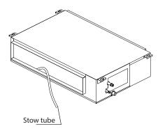
Fill the water pan with 2 liters of water. Check that the drainpipe is unhindered.
