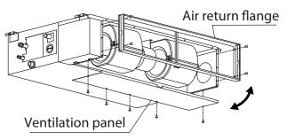
Bend the rear ventilation panel 90 degrees along the dotted line into a descending ventilation panel.(some models)
