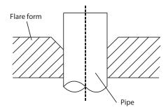
6. Place flaring tool onto the form.
