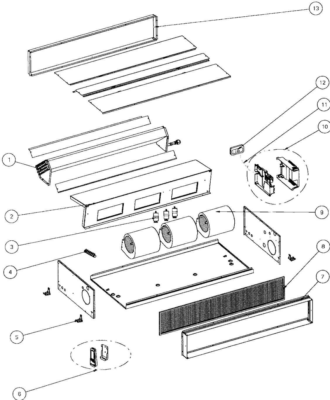
FIG.2 INDOOR UNIT ASSEMBLY – LS 065/085
