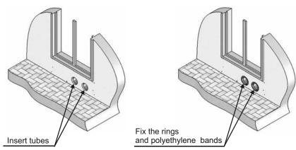
g. Connect drain tube to the nozzle of the unit and insert it through the hole  $\varnothing$ 16mm in the wall.
