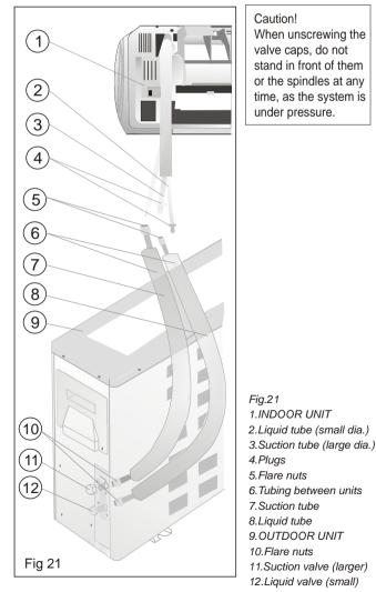
Caution! When unscrewing the valve caps, do not stand in front of them or the spindles at any time, as the system is under pressure.
