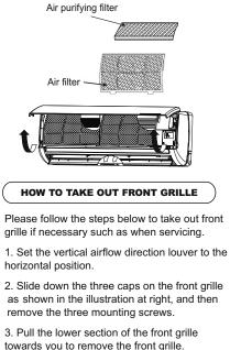
When reinstalling the front grille, first set the vertical airflow direction louver to the horizontal position and then carry out above steps 2-3 in the reverse order.
