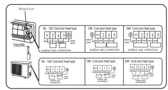
4,Secure the multiple wire cable with the cable clamps. Notes:
