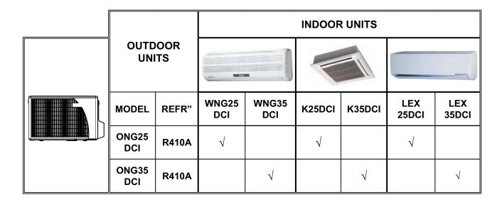
The above table lists outdoor units and WNG/LEX indoor units which can be matched together. In addition the listed outdoor units can be matched with other types of indoor units such as cassettes.
