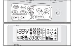
WARNING! If you do not stop pressing the keys When the screen turns black, the UBMS control unit moves into re-initialisation mode and all previously stored settings will be lost
