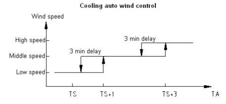
Temperature is set by remote controller (or wired controller), temperature adjustable range from 16°C- 32°C, user can adjust temperature through "temperature +" and "temperature -" button on remote controller or wired controller. Press "fan speed" button to choose fan speed among auto wind, high speed wind, medium speed wind, low speed wind.
