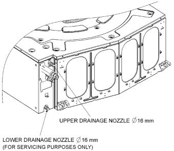
Fig. 13. Drainage connectors Ø 16 mm
