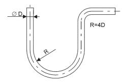
Fig. 20. The radius of curve in oil trap
