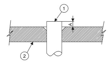
Fig. 24. Setting the tube in the flaring tool
