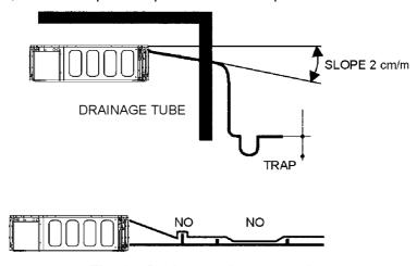
Fig. 12. Drainage tube connection
