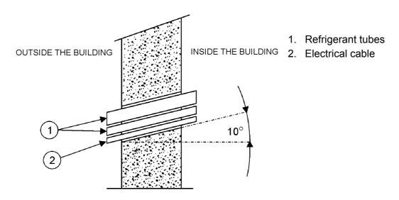
Fig. 18. Interconnecting tubing and cable between units
