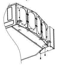
Fig. 27. Releasing screws at the bottom of the box
