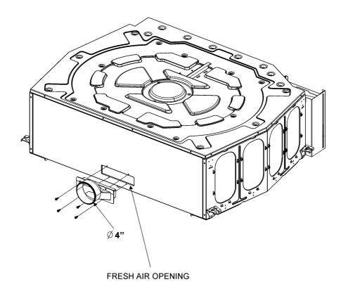
Fig. 11. Installing fresh air adapter
