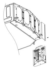
Fig. 29. Taking the box off the rail
