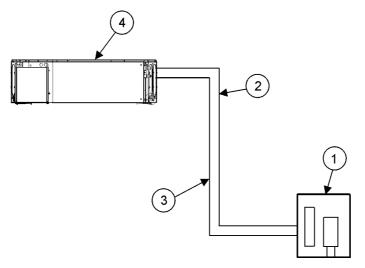
Fig. 21. Outdoor unit installed below the indoor unit
