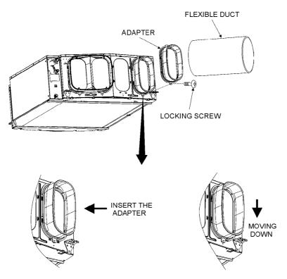
Fig. 14. Installing adapters and flexible ducts
