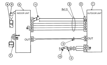
Fig. 30. Electrical wiring diagram - one-phase units (power supply to outdoor unit)
