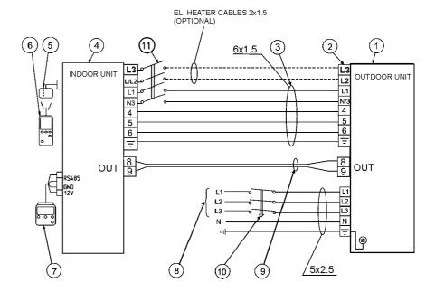
Fig. 31. Electrical wiring diagram - three-phase unit
