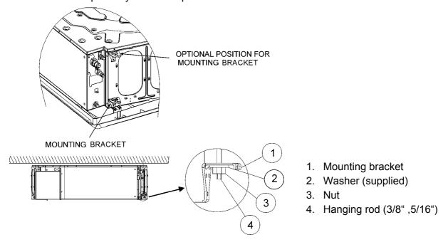
Fig. 8. Hanging the indoor unit on mounting brackets
