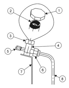
Fig. 26. Service tap for the cooling system
