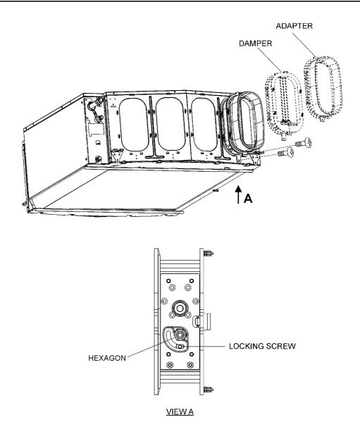
Fig. 15. Installing the manual damper
