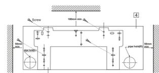
The edge of installation carton board should be more than 50mm at right and left of the wall.
