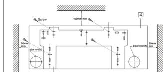
The edge of installation carton board should be more than 50mm at right and left of the wall.
