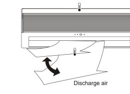
set the vertical airflow direction louver to the horizontal position and then carry out above steps 2-3 in the reverse order.
