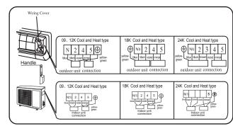
4,Secure the multiple wire cable with the cable clamps. Notes:
