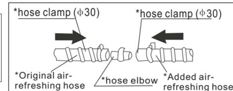
A 5m of air-refreshing hose is supplied with this equipment. You can lengthen the hose with another hose supplied by the professional installer in the installation if it is needed. Use the hose elbow and clamps to joint the smaller end (φ30) of the added hose with the original one, and then fix the other end with the interface of the propeller housing by the outdoor hose clamp (φ30). (Shown in the diagram below)
