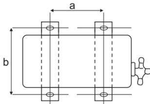
2. When installing at roof, please consider strong wind and earthquake. Please fasten the installation stand firmly with bolt or nails.
