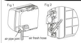
1. Joint the air pipe joint on the indoor unit
