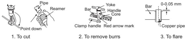
When properly flared, the internal surface of the flare will evenly shine and be of even thickness. since the flare part comes into contact with the connections, carefully check the flare finish.
