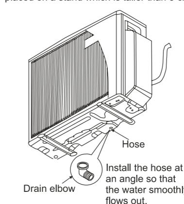
Install the hose at an angle so that the water smoothly flows out.
