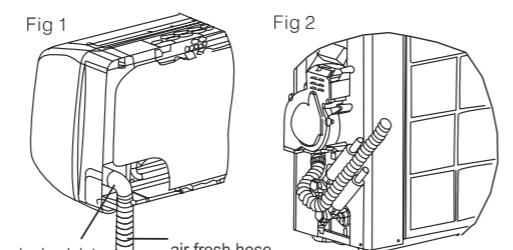
1. Joint the air pipe joint on the indoor unit.
