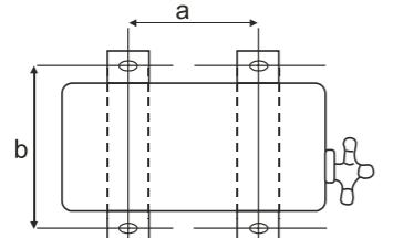
2. When installing at roof, please consider strong wind and earthquake. Please fasten the installation stand firmly with bolt or nails.
