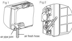
A 5m of air-refreshing hose is supplied with this equipment. You can lengthen the hose with another hose supplied by the professional installer in the installation if it is needed. Use the hose elbow and clamps to joint the smaller end ( $\Phi$  30) of the added hose with the original one, and then fix the other end with the interface of the propeller housing by the outdoor hose clamp ( \$\Phi 30). (Shown in the diagram below).
