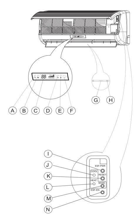
If the air-conditioner can not be operated by the Remote Control unit, it can be turned on for cooling or heating, or completely turned off, by pressing MODE button (M) on the air-conditioner. The MODE button will change the operating status of the unit between - COOLING - HEATING -STAND BY positions. Every time MODE button (M) is pressed, (J) or (L) will light up respectively, to indicate in which mode the air-conditioner operates.
