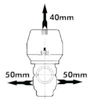
The valve must be installed horizontally to the motor above the valve axis.
