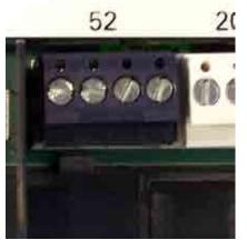
Insert plug **52** into the motor assembly
