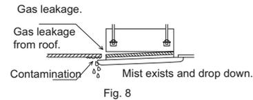
If screws are not tighten tight, problems in Fig, 8 might occur. Tighten screws properly.
