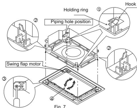
① Place the holding ring on swing flap motor side temporarily on hooks of the indoor unit. (2 pcs)
