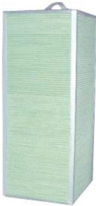
The heat recovery element is composed of flat paper and ripple paper. The thickness of flat paper is 50um. It is non-hole, water permeability but not gas permeability, which will ensure the humidity exchange and prevent the air mixture from indoor and outdoor. Meanwhile the angle between the air discharging passage and the indoor air return passage is 90degree, which can prevent air mixture further.
