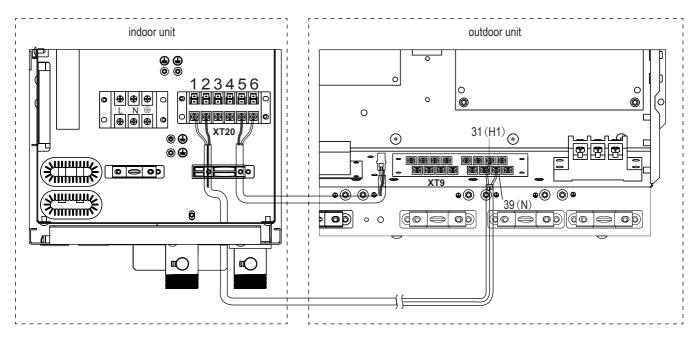
Fix the cable with cable ties to the cable tie mountings.
