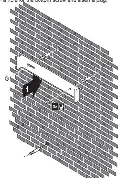
2 Fix the wall bracket to the backup heater with M4 screws.
