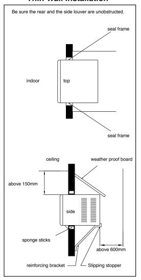
8. A stopper should be positioned at the rear to stop machine from slipping out of installation hole
