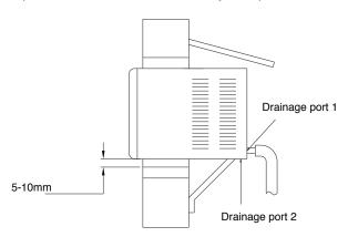
The drainage duct for KC- 15,20,25/M(E) is installed as shown in the drawing above, without drainage ports 1 & 2.
