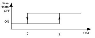
When OAT is faulty the base heater will be "ON" continuously in HEAT mode.
