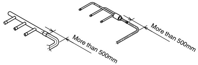
Distribution joint insulation material (supplied)
