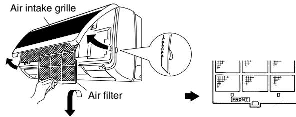
When replacing the filter, make sure that the FRONT mark is facing you.
