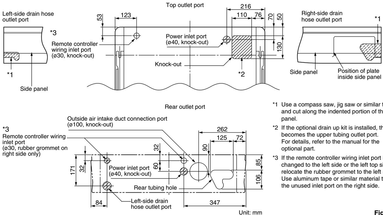
\*1 Use a compass saw, jig saw or similar tool and cut along the indented portion of the side panel.
