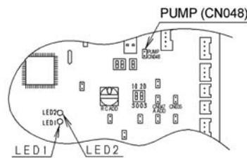
PUMP pin (CN048) is located on the outdoor PCB as shown.
