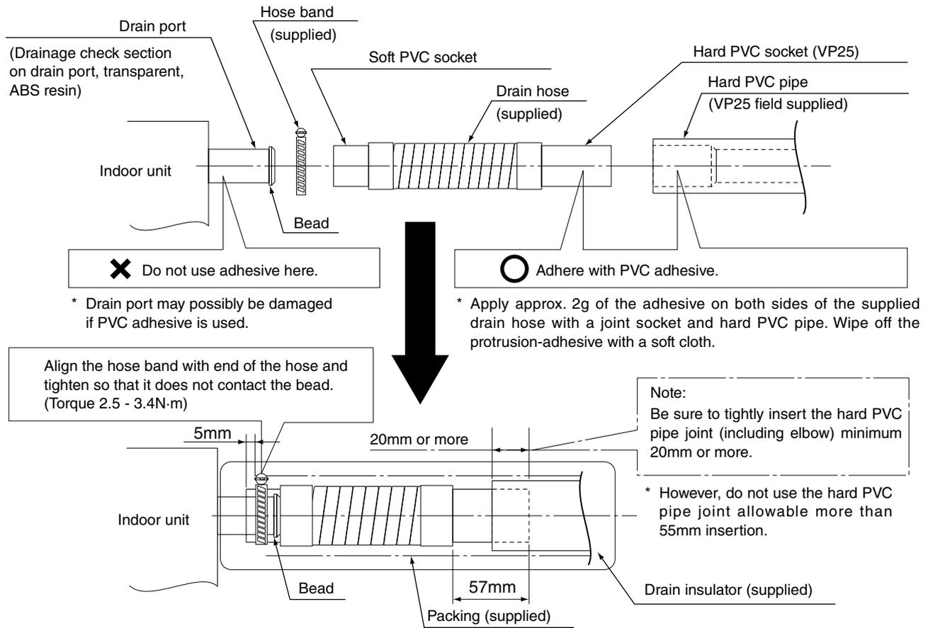
\* After checking the drainage, wrap the supplied packing and drain pipe insulator around the pipe.
