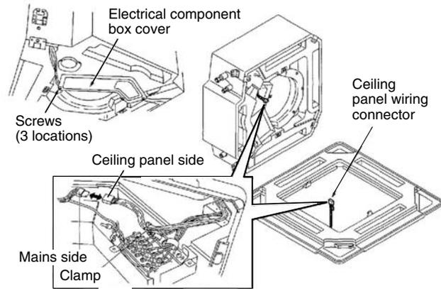
\* Pass the wiring connector through the clamp to fasten it in place, as shown in the figure.
