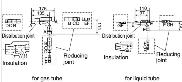
Table 1-11 Size of connection point on each part (Shown is inside diameters of tubing)
