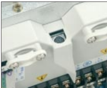
Connection board with infrared receiver terminal block.
